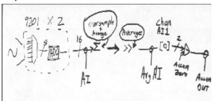
Figure 14: Analog Input System
