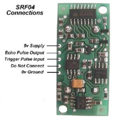
Figure 9: SRF04 Ultrasonic Rangefinder connections
