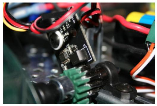
Figure 11: Gear tooth sensor with a ferrous gear cemented to the plastic Vex gear so the gear tooth senor would detect the rotation.
