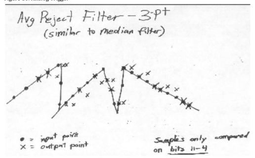
Figure 17: 3 Point Average Reject Filter
