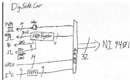
Figure 7: Digital I/O Subsystem Diagram
