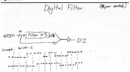
Figure 24: Digital filter diagram and example
